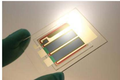
Heliatek world record cells with 12.0% efficiency on an active area of 1.1 cm<sup>2</sup>.
