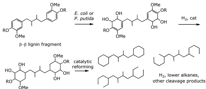
Figure 1. Schematic for converting technical lignin to alkanes via catalytic reforming
