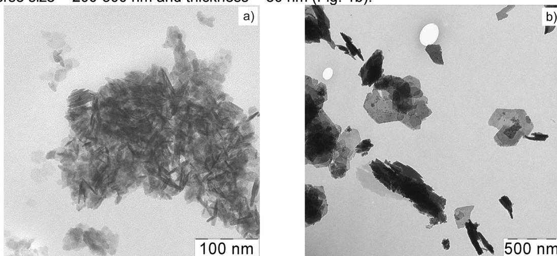
Fig. 1. Transmission electron microscopy images of feroxyhyte ( $\delta$ -FeOOH) nanoparticles synthesized under different conditions: a) in the presence of HS, b) without HS.
