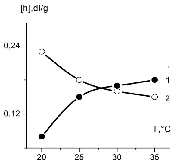
Figure 1. Characteristic viscosity of copolymer St : MA (80:20 % by weight) as the function of solution temperature. Solvents: 1 – DMFA, 2 – toluene.
